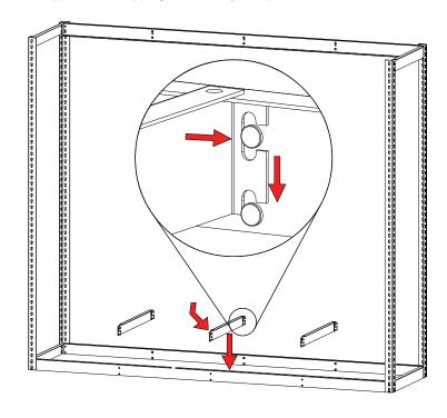
**4.** Lay the bottom steel decking (Ref. No. 6) on the shelf supports so that the front and back edges overlap the front and back shelf supports.
