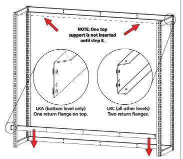
NOTE: The two LRA supports at the bottom have no return flange on the bottom edge, while the LRC support have a return flange at both the top and bottom.
