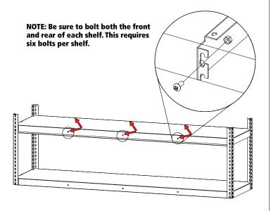
NOTE: Bolts are not needed to secure the deck supports on the bottom shelf because it rests on the floor. All other levels require these bolts to achieve maximum load capcities.
