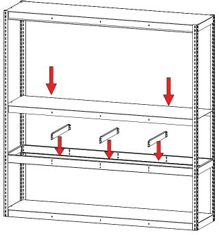
NOTE: Every fourth slot in the uprights has a flat top to help visually align the supports.
