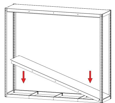
**5.** Attach shelf supports at the next desired shelf level. Once the shelf supports are in place, attach three front-to-back center supports as you did in step 3. Lower the steel decking into place, as described in step 4.
