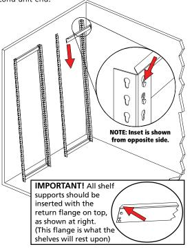
**2.** Next, connect the two unit ends with two LRA left-to-right shelf supports (Ref. No. 3) at the bottom and one LRC left-to-right shelf support (Ref. No. 4) at the top, temporarily leaving off one of the top left-to-right supports.
